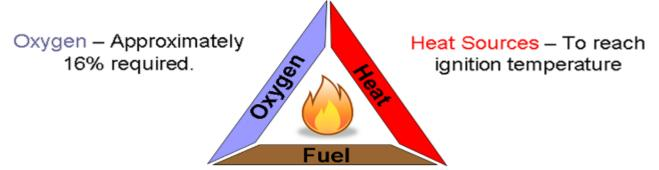
Fuel - Gases, Liquids, Solids (Bulky - Dust)
